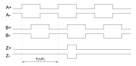
Fig.5.5.: Time diagram with differential TTL quadrature signal
