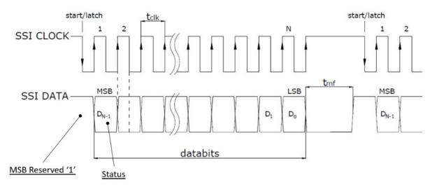
Fig.5.4.: Time Diagram for the SSI02 interface
