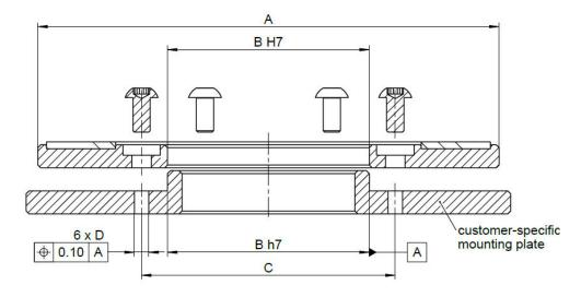
Fig.4.2.: Rotor (GAR) mounting using ID sliding fit
