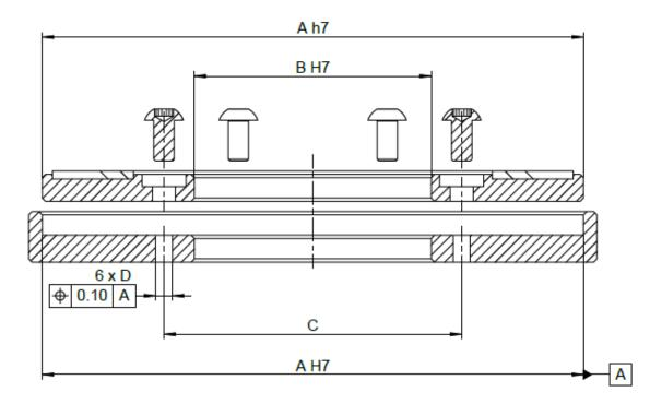
Fig.4.3.: Rotor (GAR) mounting using OD sliding fit
