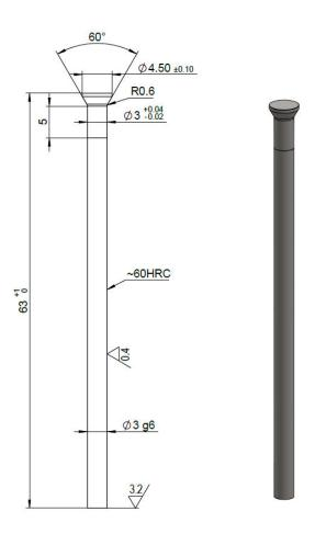
Fig.11.2.: Dowel pin DP-3g6-63 dimensions
