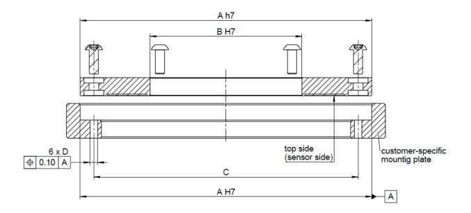
Fig.4.3.: Stator (GAS) mounting using OD sliding fit
