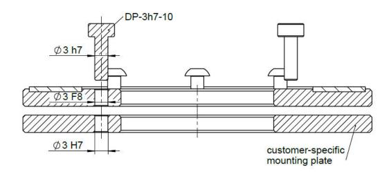
Fig.4.6.: AMR Dowel-Pin mounting
