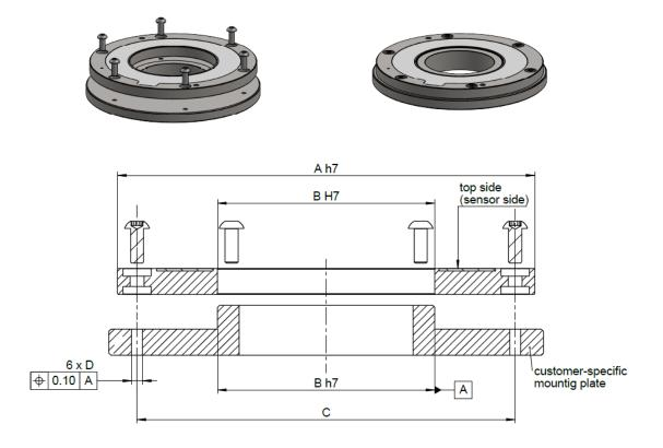
Fig.4.1.: Stator (GAS) mounting using ID sliding fit
