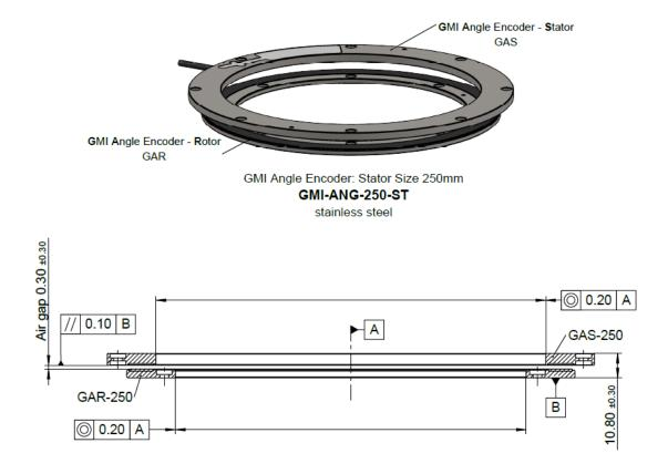
A ... axis of rotation max. total runout GRS + GAR = 0.20mm / GAS + GAR 0.20 A Dimensions are mm.
