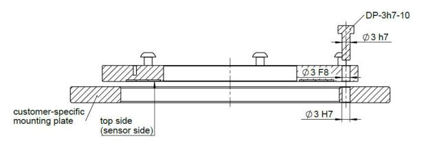
Fig.4.5.: AMH Dowel-Pin mounting
