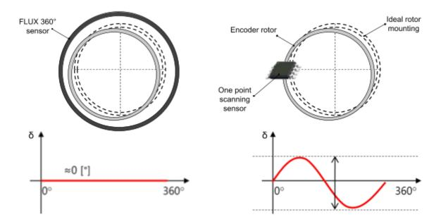
Sensor geometry causes FLUX encoders to inherently average out eccentricity across the circumference of the rotor, resulting in significant reduction in eccentricity error. However, a sensor with a "one-point" scanning capability will exhibit eccentricity errors [ $\delta$ ] over a complete rotation in the form of a sinusoidal wave.
