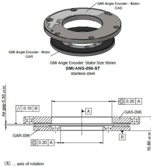
max. total runout GRS + GAR = 0.20mm f GAS + GAR 0.20 A Dimensions are mm.
