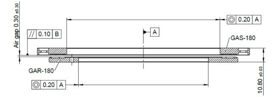
A ... axis of rotation max. total runout GRS + GAR = 0.20mm / GAS + GAR 0.20 A Dimensions are mm.
