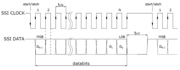
Fig.5.2.: SSI01 time diagram
