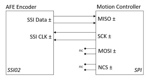
Fig.5.3.: Interfacing the SSI02 to the SPI master
