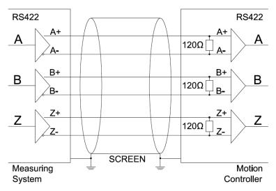
Fig.5.6.: Recommended electrical connection and buffering
