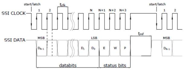
Fig.5.1.: SSI00 time diagram
