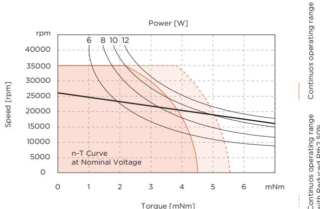
Example: Power diagram for rated values at continuous operation.
